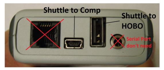
There is only one cable, but 2 port options, for the shuttle. When you want to plug the shuttle into the computer, you place the mini-B USB cable into the (Shuttle to Comp) port. When you want to plug it into the HOBO you use the (Shuttle to HOBO) port.
