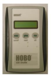
The shuttle is the ONLY way you can communicate with the HOBO weather station - so be nice to it. The top of the shuttle looks like this:
