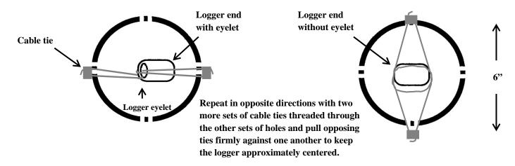
Figure 3. Protective housing for sea surface temperature data logger.
