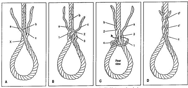
An eye splice forms a permanent loop in a line; it may be made around a thimble to guard against chafe (such as occurs on an anchor line), or around an eyelet as part of running rigging.
