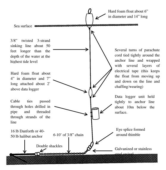
Figure 1. Sea surface temperature data logger anchor system.
