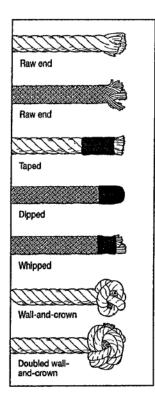
Ends of a three-strand or braided line can be taped, dipped in a sealer or whipped to prevent unlaying. Also shown is the wall-and-crown, a good-looking finish that combines two simple knots, and the manrope knot—a doubled walland-crown.
