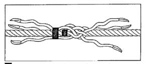
3 Working with the three free strands, remove temporary seizing from around the other rope and splice the strands into it by tucking the loose strands over and under successive strands from right to left against the lay of the rope. When first tucks have been made, snug down all three strands. Then tuck two or three more times on that side.
